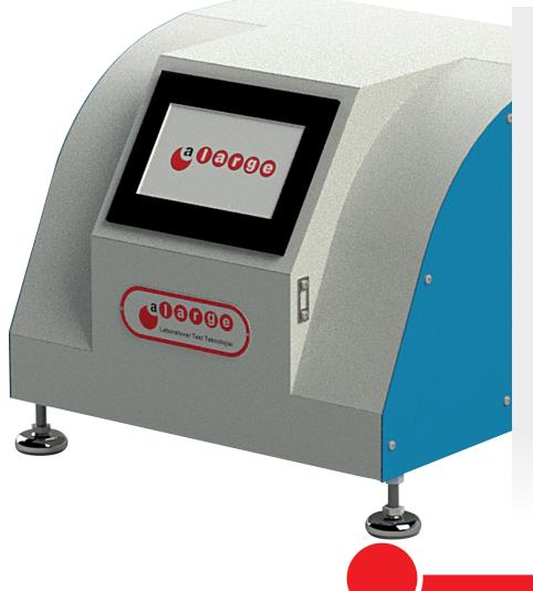
It is a method for testing joints, fittings, pipes etc. under a vacuum leak test for thermoplastic piping systems. It applies to piping systems based on thermoplastic pipes designed for use in hot and cold water pressure applications.
